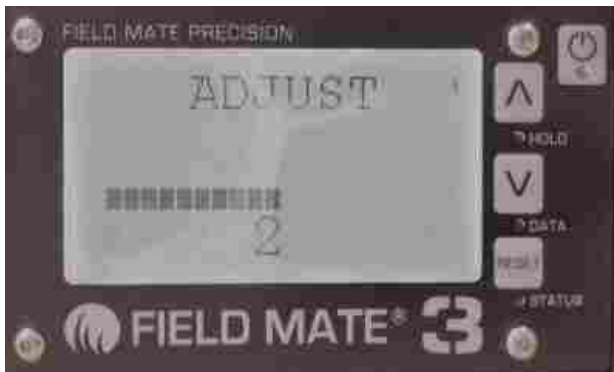
Holding the arrow key
