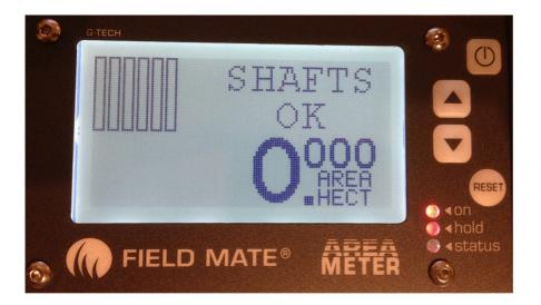
Main Screen ... Bar Graphs move as shafts rotate. ...Press RESET to zero area.
